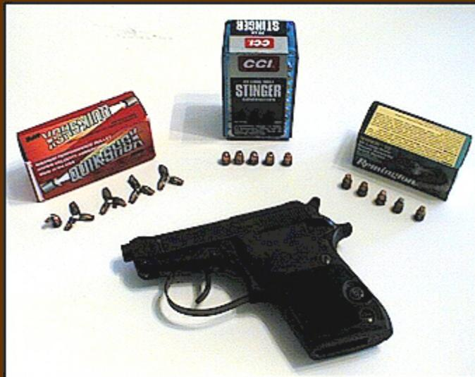
Figure 1. Recovered bullets which represent observed terminal performance. Clockwise from top: CCI Stinger hollowpoint (all bullets failed to expand), Remington Viper truncated cone, Beretta M21A test gun and MPB Quik-Shok prefragmented-hollowpoint (one bullet failed to fragment).
